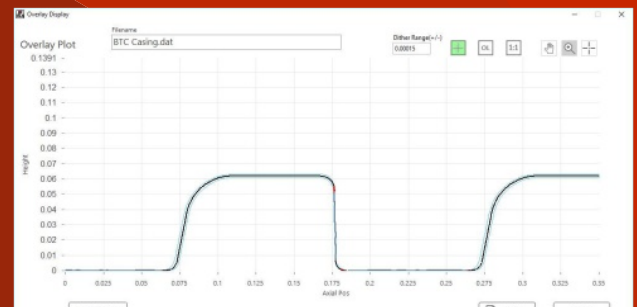
OVERLAY COMPARISON: COMPARES THREAD OVERLAY TO ELECTRONIC THREAD MOLD
